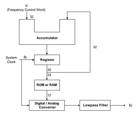
A DDS frequency synthesizer consists of a phase accumulator, a lookout table (ROM or RAM), a Digital-to-Analog Converter (DAC), and a Lowpass Filter (LPF). The amount in a phase accumulator is controlled by the frequency control word (K), which will be added by 1 after each system clock cycle(=1/fs). The output of the accumulator is used to position the data in the Table ROM (or RAM). The digital data will then be converted into a smooth analog waveform after passing through the DAC and LPF.
